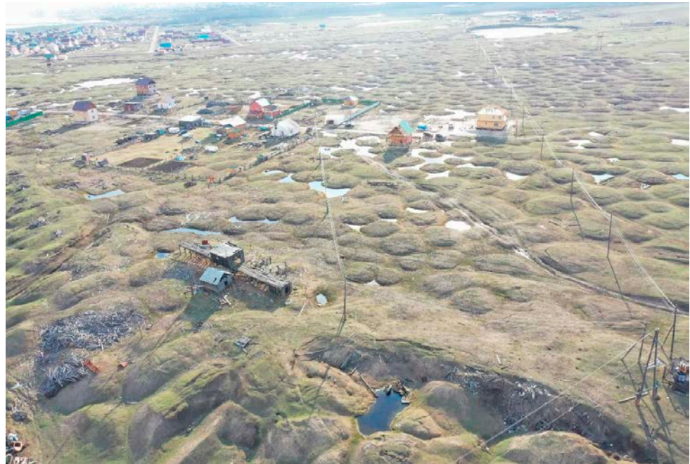
Figure 2. Thermokarst microrelief formed as a result of the thermokarst processes (permafrost degradation) in the study area.
